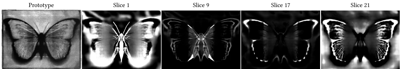
Fig. 5. Front view of the printed planar prototype of the Butterfly scene. The prototype is printed with 24 slices. We show a visualization of absorption coefficients of slice 1, 9, 17, and 21.
