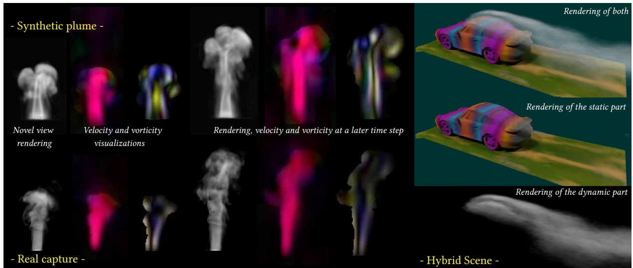
Fig. 1. Renderings and visualizations of fluid reconstructions. Using sparse image sequences, we learn continuous radiance and velocity fields to represent fluid scenes. We can handle synthetic and real scenes (on the left) as well as hybrid scenes (on the right). Our method supports arbitrary obstacles and unknown lighting conditions flexibly.
